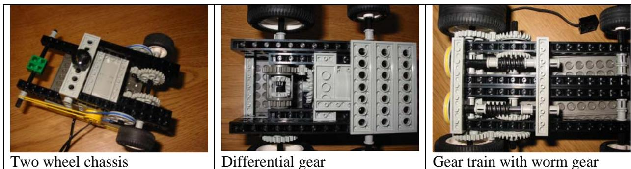
*Figure 4: Sample chassis design undercarriages*
